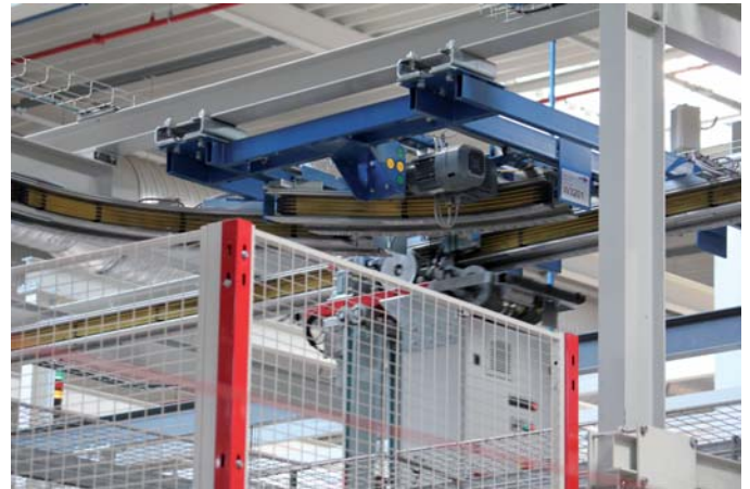
IPT® (Inductive Power Transfer) and electric monorail conveyor from Conductix-Wampfler
