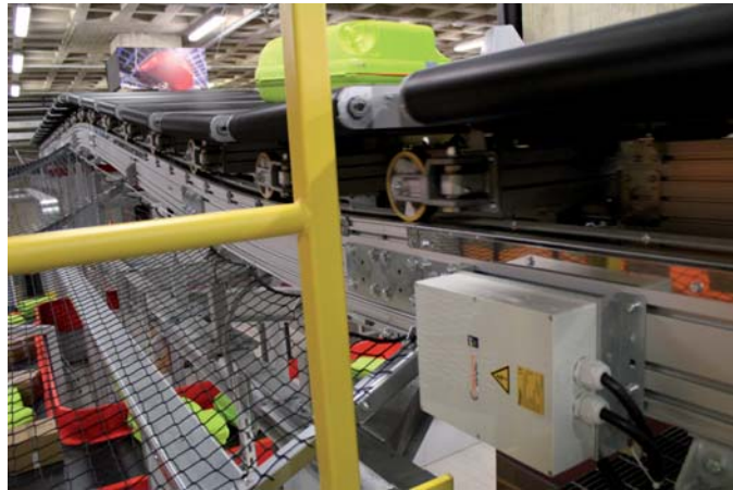
IPT® (Inductive Power Transfer) and electric monorail conveyor from Conductix-Wampfler
