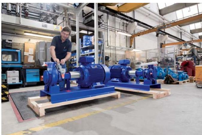
*Final assembly steps of a KSB pump*
